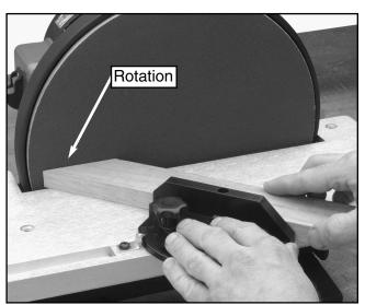
Figure 9. Mitering with gauge angled.
